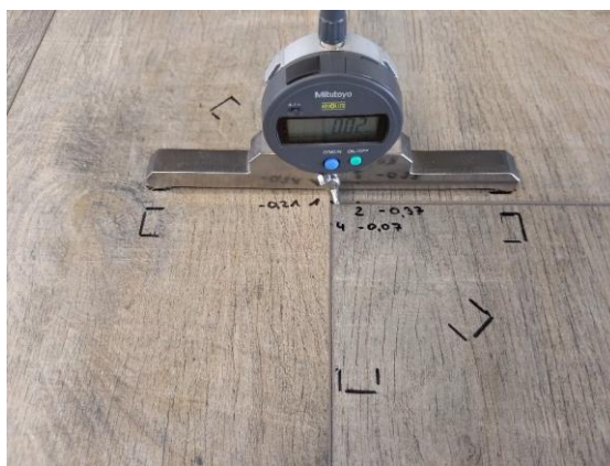
Figure 5: Example showing the markings for the supporting feet of the measuring device
