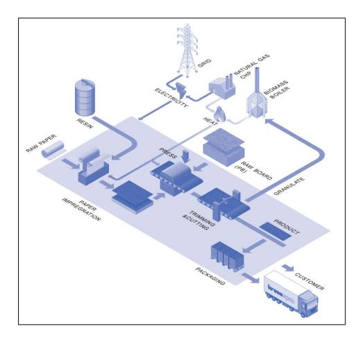
Raw particleboard is produced by taking recycled wood chips, removing all contaminants (which are sent for further recycling) and combining this with sawdust, resin, wax and hardener. This material is then pressed into long sheets of particleboard of the desired thickness. The thermal energy is derived from biomass residues and electrical energy is derived predominantly from on-site generation with natural gas as fuel.
